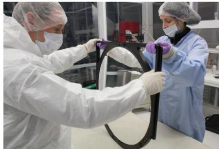
Figure 1: Checking filter N964 following installation into its mounting frame, in the Blanco cleanroom. Left to right: Roberto Tighe and Nicole David. (Image credit: Freddy Muñoz/NOAO/AURA/NSF.)
