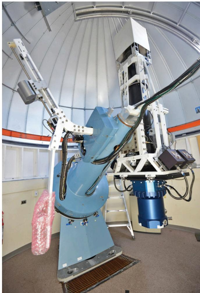
The USNO Robotic Astrometric Telescope. The white top box serves as dust protection and contains the motorized lens cover (206-mm entrance pupil aperture). The blue dewar contains four big CCDs (111 million pixels each) and has a 300 mm dewar window that also serves as the bandpass filter. Note the moving counterweight on the left arm, which is needed to balance the changing weight of LN<sub>2</sub> fill of the dewar. (Image credit: Norbert Zacharias/USNO.)
